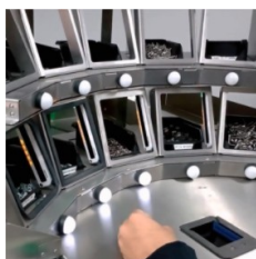
Pick Count Mesa com sistema inteligente de picking by light
